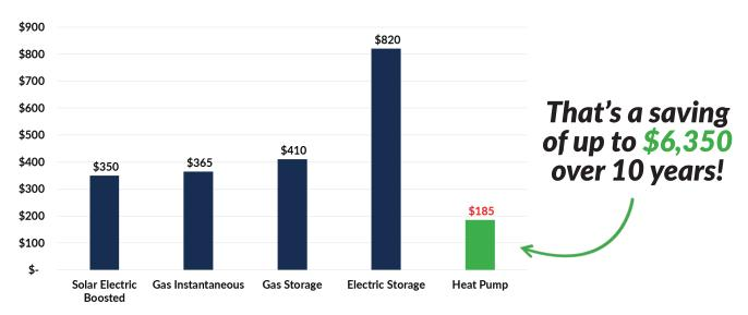
Data sourced from Sustainability Victoria's Hot Water Running Costs 2020 and compares running costs of a 5.5-star gas storage system, 7-star gas instantaneous system, electric storage off-peak system, high-efficiency solar gas boosted system, high-efficiency solar electric boosted system, high-efficiency hot water heat pump on off-peak tariff.
